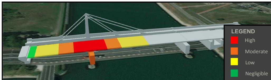
**Fig. 1.** The 3D bridge model appears with traffic light colour sets as the colours express the risk value of the damaged bridge components.
